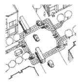
The pedestrian walkway material should be firm, planar, and slip-resistant. Concrete is the preferred walking surface. A different look can be achieved by using stamped concrete or concrete pavers, which are available in a variety of colors and shapes; however, jointed surfaces may induce vibration, which can be painful to some pedestrians. They can also be used on the top of raised devices.
