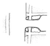
Chokers can have a dramatic effect by reducing a two-lane street to one lane at the choker point (or two narrow lanes), requiring motorists to yield to each other or slow down. In order for this to function effectively, the width of the travelway cannot be wide enough for two cars to pass: 4.9 m (16 ft) is generally effective (and will allow emergency vehicles to pass unimpeded). This kind of design is usually only appropriate for low-volume, low-speed streets.
