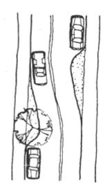
Diverting the Path of Travel. Shifting a travel lane has an effect on speeds as long as the taper is not so gradual that motorists can maintain speeds. For traffic calming, the taper lengths may be as much as half of what is suggested in traditional highway engineering.
