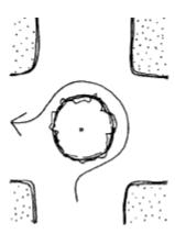
Mini-circles are an intersection improvement as well as a traffic-calming device and can take the place of a signal or four-way stop sign. Many unwarranted four-way stop signs are installed because of the demand for action by the community.
