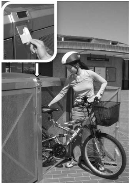
Figure 4. Electronic Bike Lockers at North Berkeley BART Station (Insert shows smart card used to access lockers)
